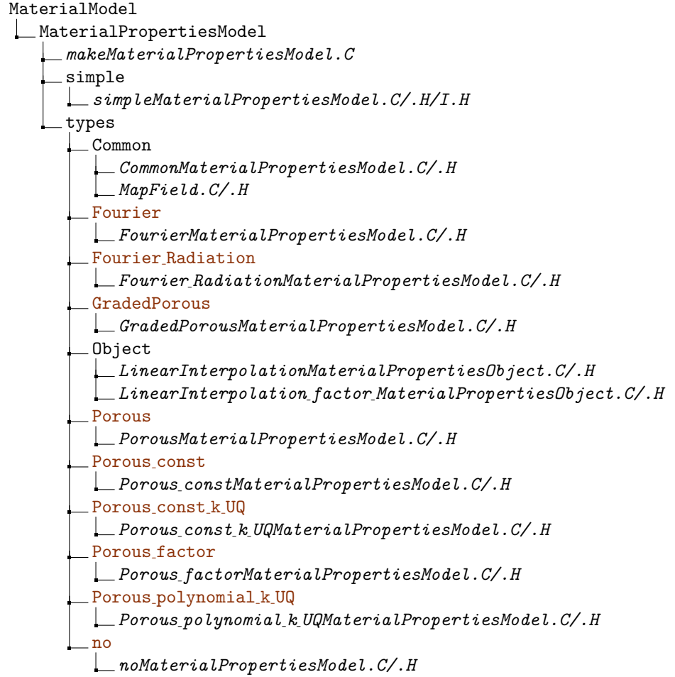
Figure 2.7. MaterialProperties model architecture
