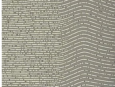
FIGURE 2. Undulating electrode and dielectric layers.
