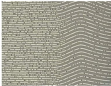
FIGURE 2. Undulating electrode and dielectric layers.
